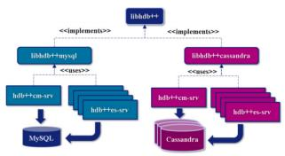
Figure 1: HDB++ Device Servers design.
