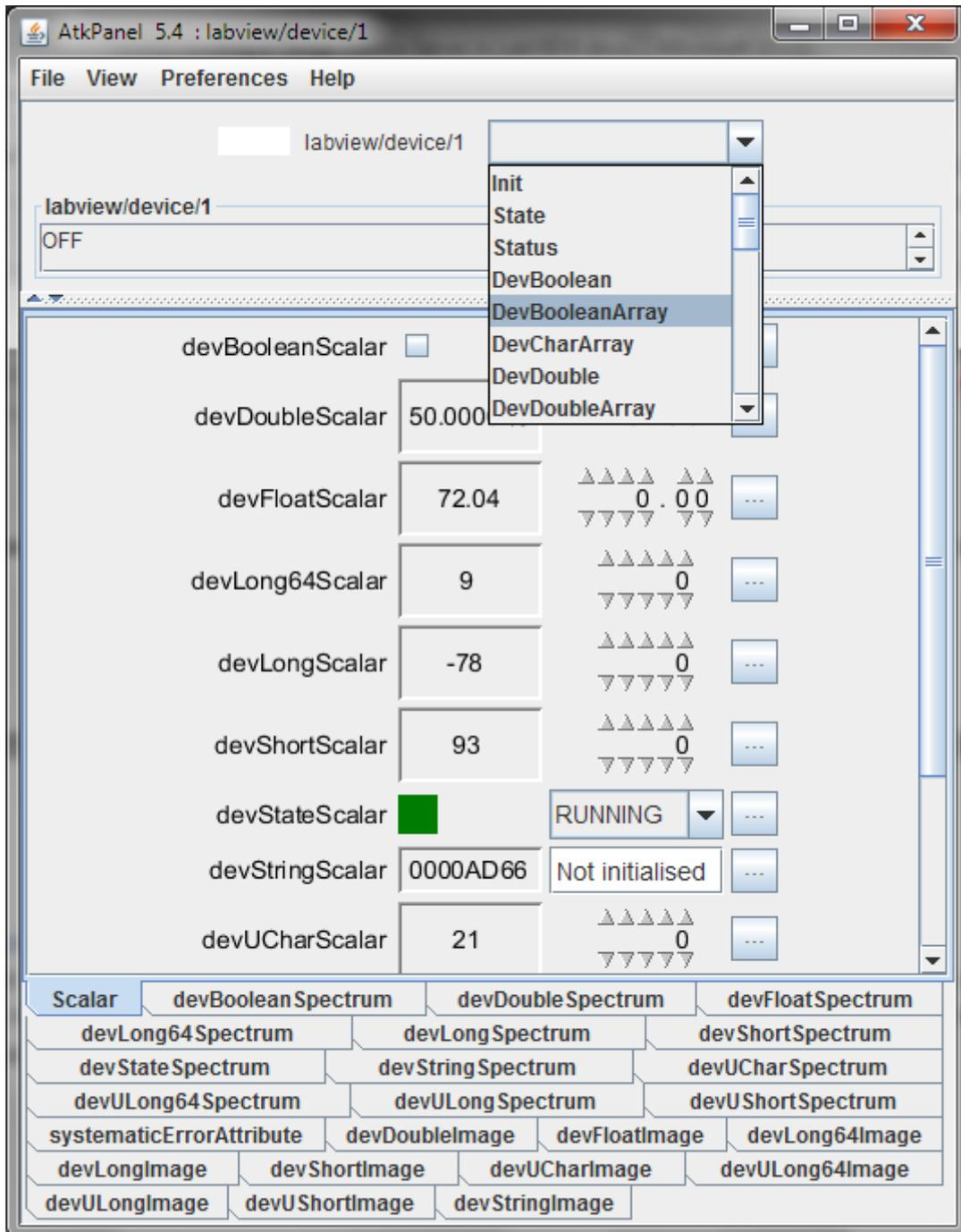
The binding also comes with a set of unit tests you can use to test the device and evaluate its performances and stability. Don't hesitate to launch a couple of them in order to estimate the responsiveness of the device under heavy load (e.g. play with the **devDoubleScalar** knob while the device is responding to client requests). Launching the **ClientForSingleDeviceDServer\_[03,04].vi** generates something like 1000 requests/s on a i7 laptop.
