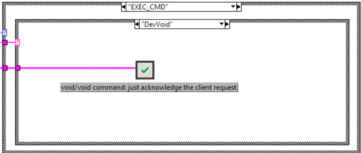
Please note that, whatever is the request type, the `_DServerRequestAcknowledgement.vi` can be used to send an error to the client - e.g. invalid argument, value out of range, etc.
