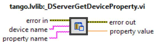
Device properties are usually read upon reception of an "Init" command request. Here is an example:
