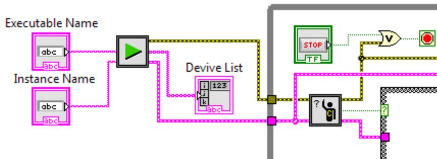
A client request is primarily identified by its type: `EXEC_CMD`, `READ_ATTR` or `WRITE_ATTR`. It also contains the device name and the name of the command or attribute to which it applies. Using case structures, it then becomes straightforward to identify and reply to client requests:
