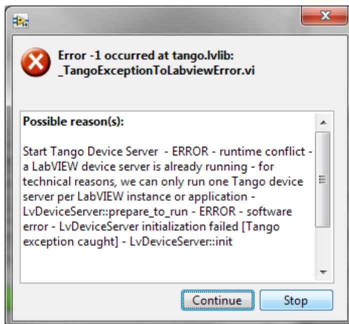
Don't be confused. Running several devices into the same device-server is supported – see the *examples.lvlib::MultiDeviceDServer.vi* for an example. What is not supported is running two device-servers into the same LabVIEW session (or application). This is also a Tango kernel constraint inherited from the C++ implementation – i.e. running two device-servers into the same process is not supported (which clearly makes sense).
