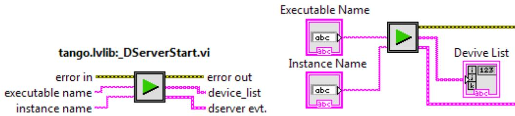
The `dserver evt.` terminal of the `_DServerStart.vi` is then injected into the `_DServerEventHandler.vi` which is itself running into an infinite while loop. The `_DServerEventHandler.vi` is the unique entry point of any *client request*.
