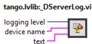
The logging level is controlled by the **tango.lvlib::\_LoggingLevel.cti** (typedef) .
