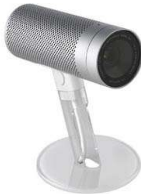
Apple iSight – example of a low cost ccd camera interfaced with Ieee 1394
